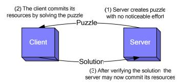
Fig. 1. Principle of the client puzzle protocol
