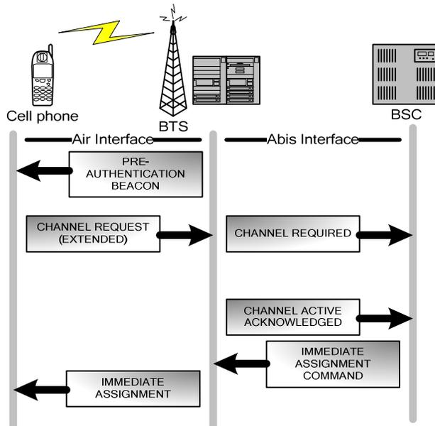
Figure 5. DOS-resistant channel assignment process in GSM
