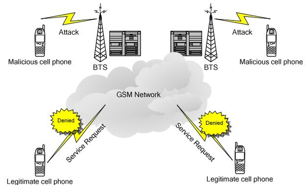
Figure 4. Denial of service attack in a GSM network
