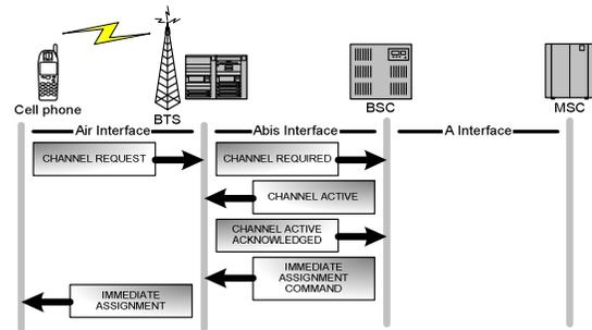
Figure 3. Channel assignment process in GSM
